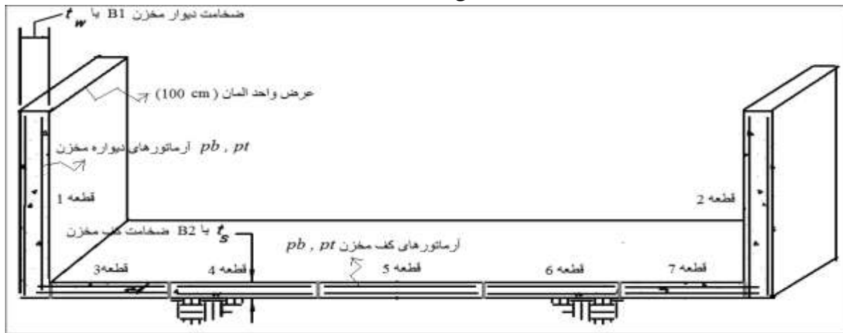
Fig 2. Schematic figure of the section of the cylindrical tank and its segmentation
