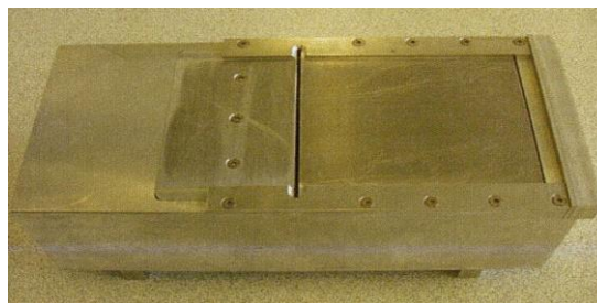
Fig 4. The orifice used in the experiment by Alsaydalani (2010)
