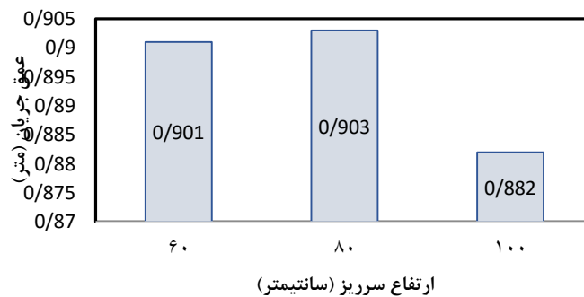
Fig 21. Comparison of the depth of the flow created on the lateral weir of the sharp edge with different heights and considering the height parameter of the crown weir
