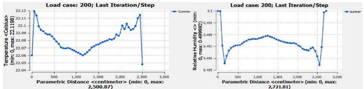
Fig. 56 and Fig.57. Levels of fluctuations in the temperature with the tolerance of 0.08 degrees centigrade on the left while on the right hand we can observe the fluctuations in humidity with the tolerance of 0.003%.
