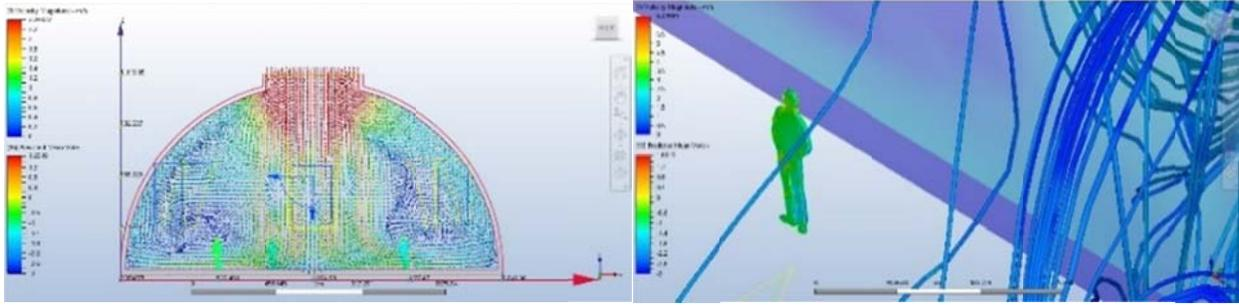
Fig. 46 and Fig.47. The airflow pattern and the air temperature is shown on the right image and the PMV index with a desirable high degree is shown in the right image.
