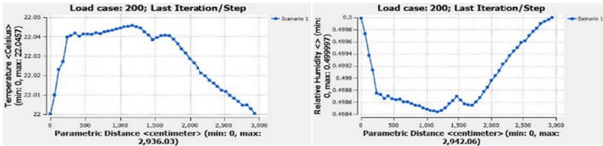
Fig. 11. and Fig. 12. Diagram of the fluctuations in the exhibition in the exhibition space is shown in the left image and the chart of changes in humidity is shown in the right image.
