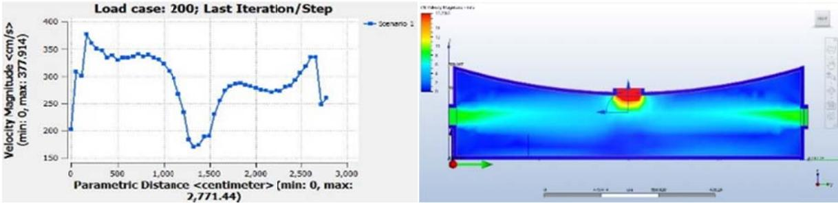
Fig. 9. and Fig. 10. diagram of the wind speed in the exhibition is shown in the left image and a section of the exhibition space length and the amount of air speed near the air intake and exhaust frames in the right.
