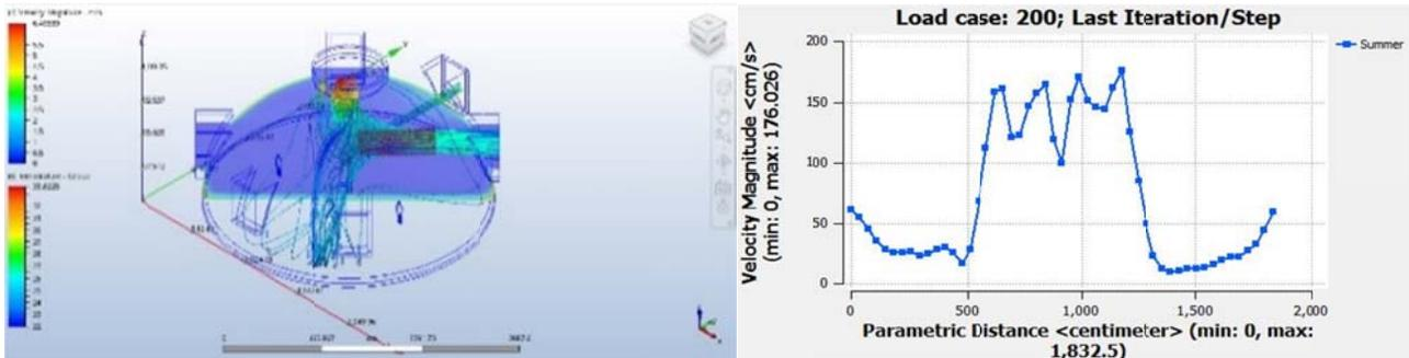
Fig. 42 and Fig. 43. Type and pattern of the airflow is shown in the left image while on the right image the changes in the airflow speed is indicated with a 1.4 m/s tolerance.
