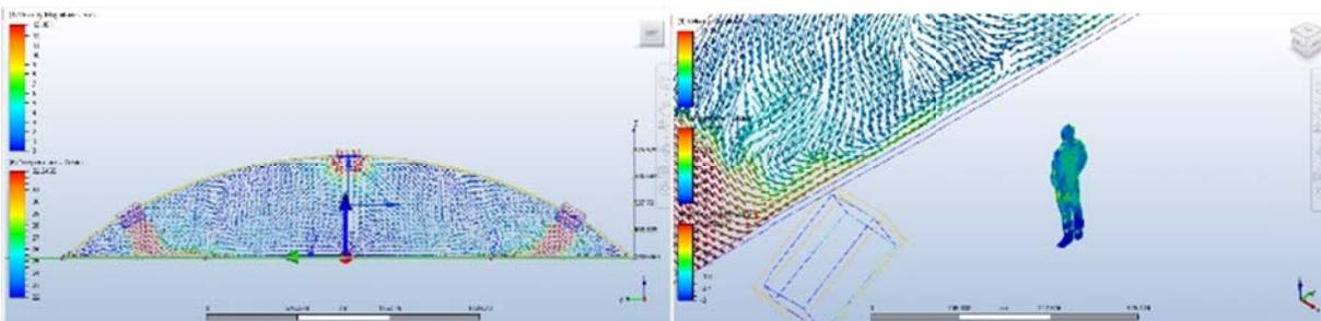
Fig. 58 and Fig.59. The quality of air movement is evident on the left image while the PMV thermal welfare index on the model shows that the cold air is located at the bottom of the model.
