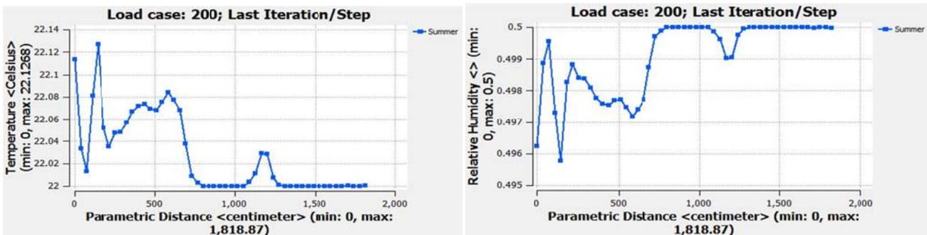
Fig. 44 and Fig.45. The levels of fluctuations in the exhibition space temperature is indicated with a 0.13 centigrade tolerance while in the left image while the amount of fluctuations in the humidity is indicated.
