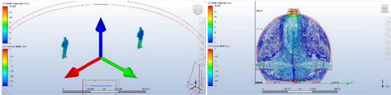
Fig. 40 and Fig. 41. The PMV index is shown in the left image and on the right image the airflow pattern is shown.
