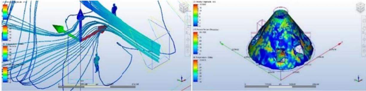
Fig. 17 and Fig 18. Airflow pattern and the extent of thermal comfort based on the PMV index is shown on the right image and the temperature dispersion in the environment is shown in the left image.
