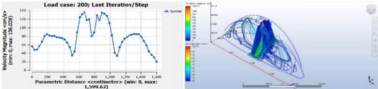
Fig. 30. The airflow speed in the length of greenhouse is indicated in the left image and the air flow type and pattern is shown in the right image.
