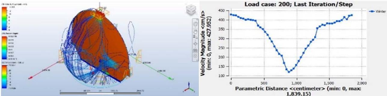
Fig. 36 and Fig. 37. Type and pattern of the airflow is shown in the left image while on the right image the changes in the airflow speed in the exhibition is indicated.
