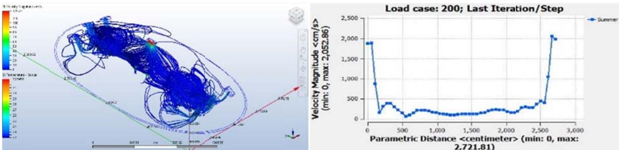
Fig. 54 and Fig. 55. The quality of air movement with the maximum speed of 2 meters per second is observable on the left hand while on the right side changes in speed is indicated which is in its maximum amount in the in take frames which increases to 0.5 meter per second.
