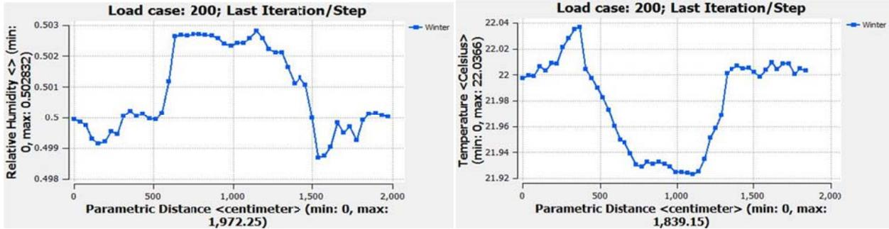
Fig. 38 and Fig. 39. The rates of fluctuations in the humidity of exhibition space is shown in the left image while the amount of fluctuations in the air temperature is indicated.
