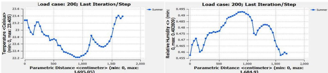
Fig. 31. and Fig.32. Fluctuations in the air temperature levels in the length of greenhouse is shown in the left image while the changes in the rates of air humidity is shown in the right image.
