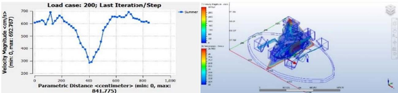
Fig. 23 and Fig. 24. Fluctuations in the air current speed in the 10 meter radius of the greenhouse is observable on the left while the type and pattern of the airflow current is shown in the right.
