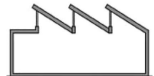
Fig. 6. Section of the sawtooth (Asdrubali, 2003)
