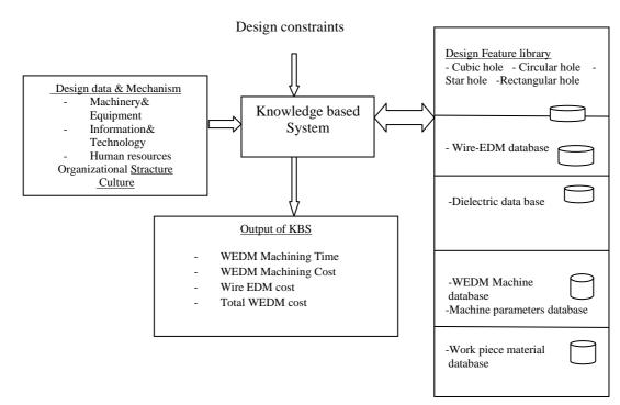
Figure4. Input, Output, constraint and databases of IKBS
