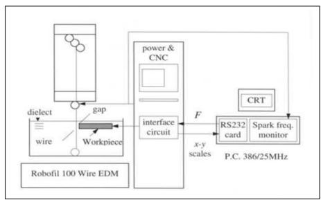
Figure2. Schematic diagram of process in WEDM
