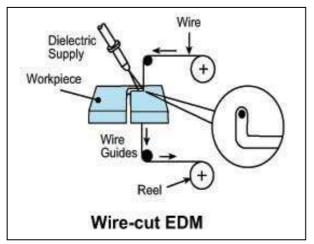
Figure1. Schematic diagram of WEDM
