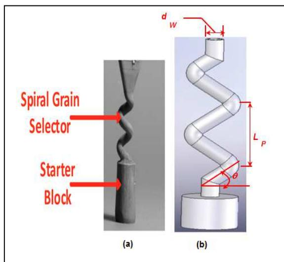
Figure 1(a). Illustration image of single crystal grain selector [13] (b). 2D grain selector with parameters
