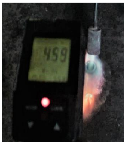
Figure 6. Bush heating up to 459 °C by direct flame
