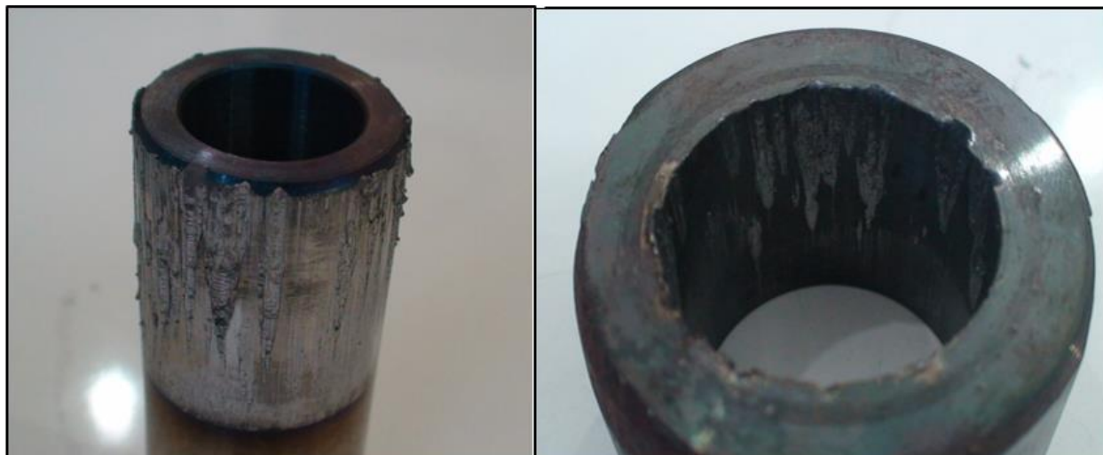
Figure 13. Surface quality of parts disassembled by thermal method
