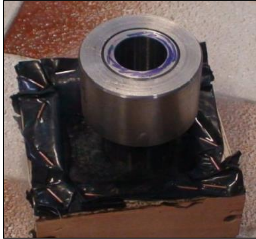
Figure 11. Placement of the axle side of the set inside the LN
