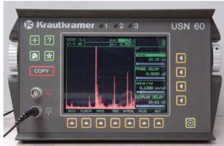
Figure 4: Ultrasonic device for tracking discontinuity
