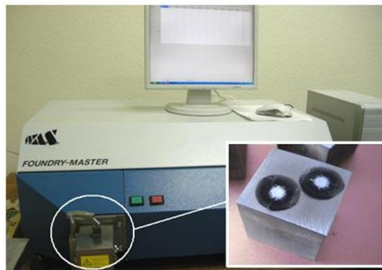
Figure 5. A quantum device to detect alloy elements
