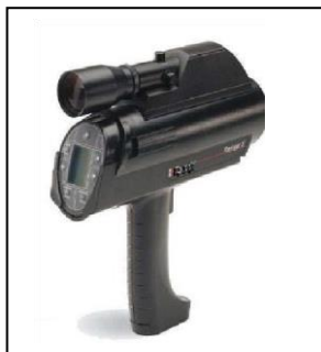
Figure3. The schematic view of a non-touch laser thermometer
