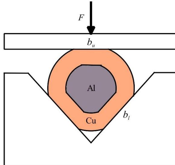
Figure 9. The contact lengths of the bimetallic rod with the die surfaces
