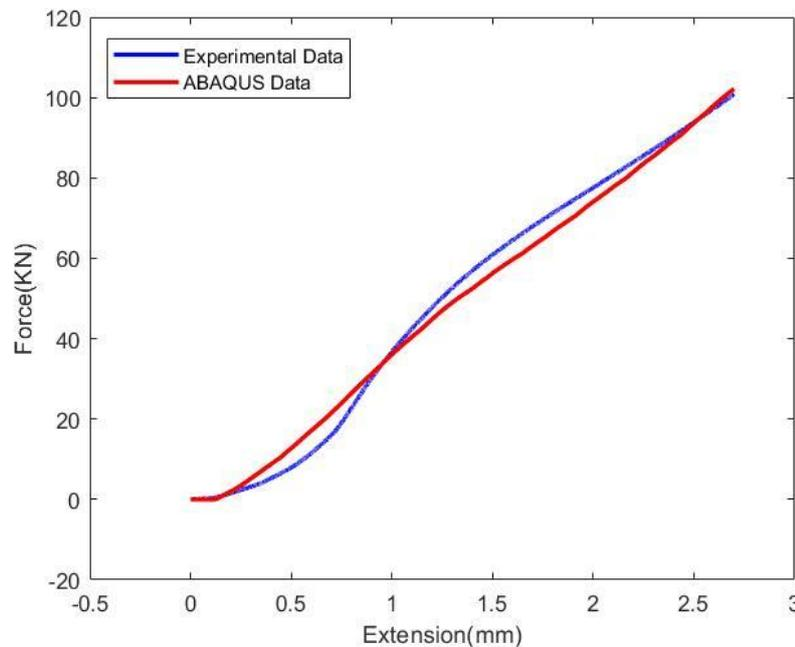
Figure 10. Experimental and numerical diagrams of the change in the forming force according to the press stroke
