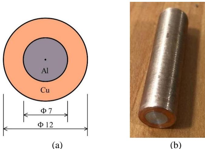
Figure 5. a) Dimensions of cross-section b) bimetallic rod sample
