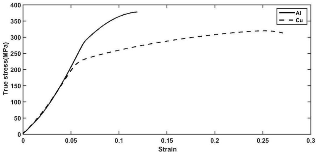
Figure 4. True stress-strain diagram of aluminum series 10 50 and copper Cu-ETP R250
