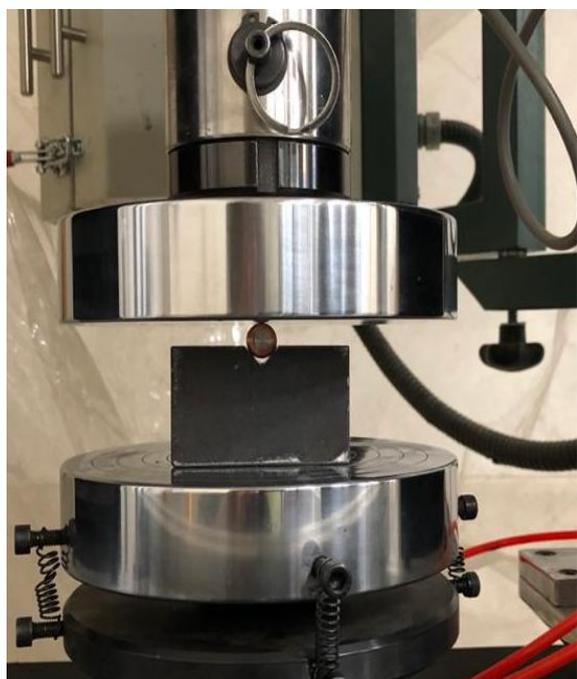
Figure 6. The process of lateral compression of the bimetallic rod at the start
