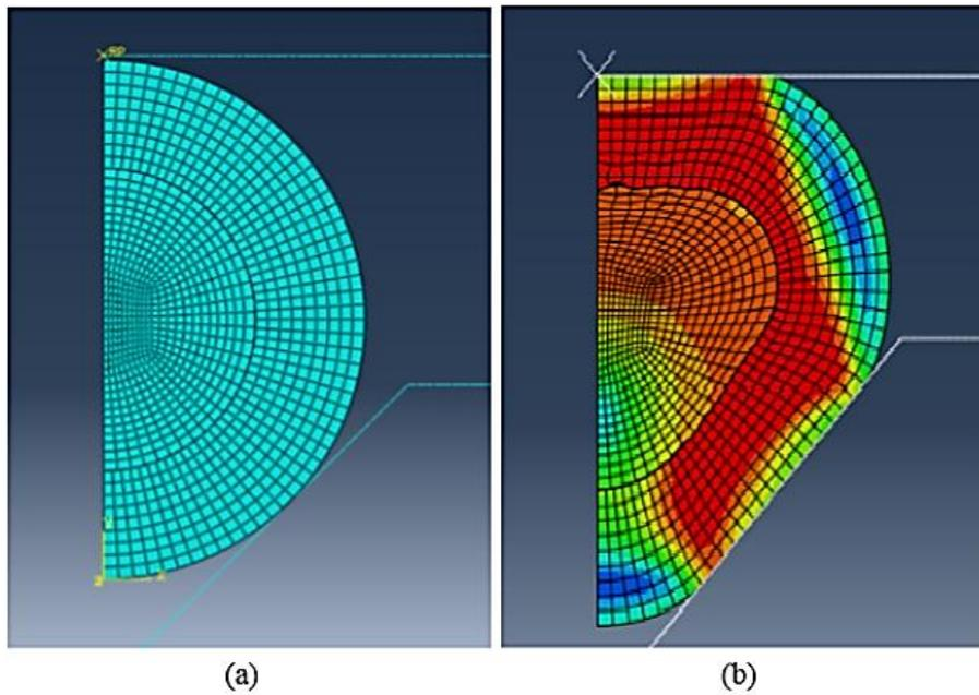
Figure 8. a) FE simulation model, b) deformed mesh after the implementation of the process at press stroke 2.7 mm
