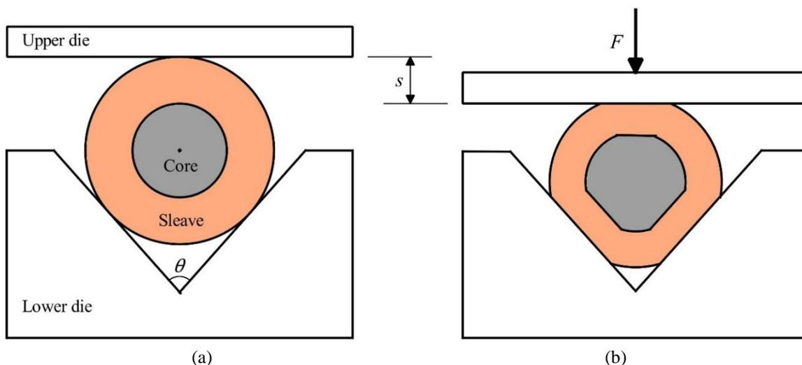
Figure 1. The process of the plane strain compression of the bimetallic rod between the flat and V-shaped dies : a) before deforming, b) after deforming
