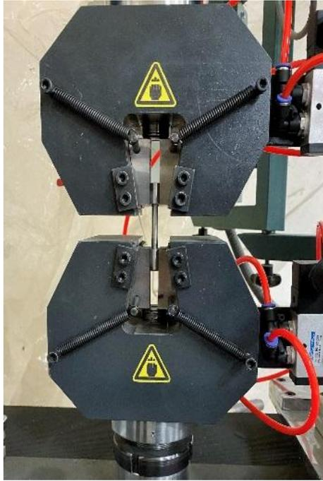
Figure 3. Aluminum specimen in the tensile test machine
