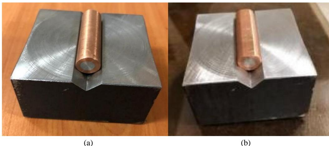
Figure 7. Placing the bimetallic rod on the lower V-shaped die, a) before b) after applying the compression force
