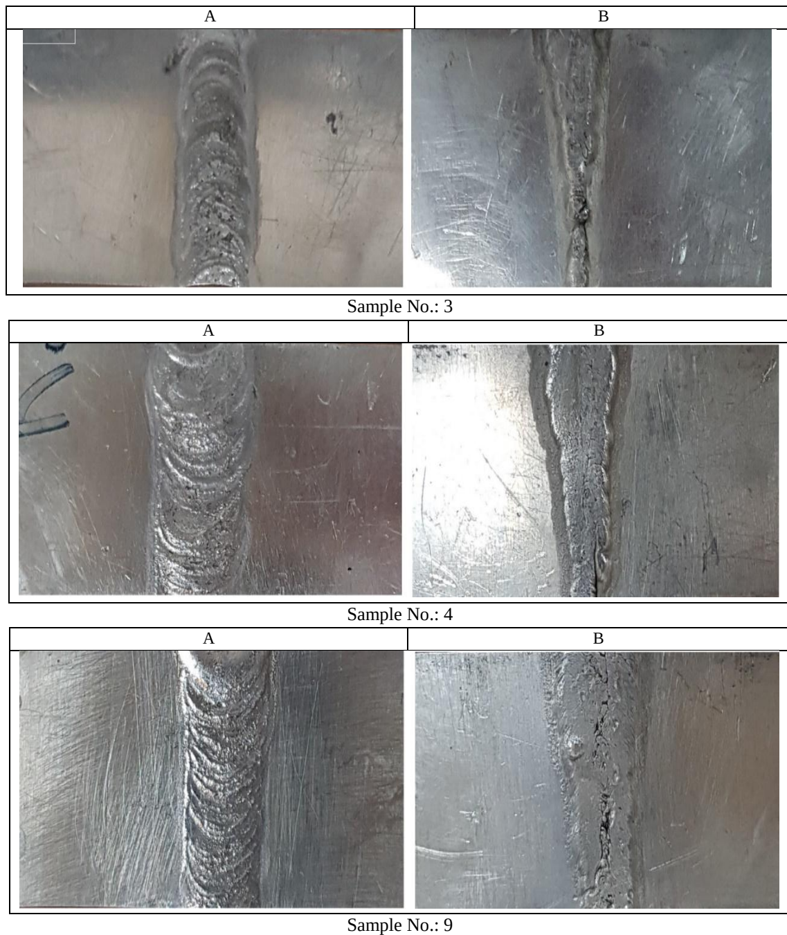
Figure 3. A and B show the top surface and the root of the weld appearance in the confirmed parts after the VT
