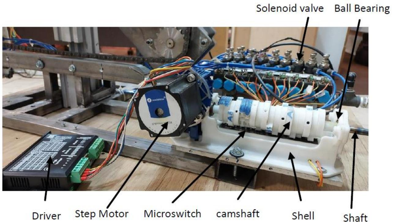
Figure 4. The developed mechanical system to control microswitches and solenoid valves. As can be seen, the components of the proposed system consist of a driver, step motor, microswitch, camshaft, shell, and shaft.
