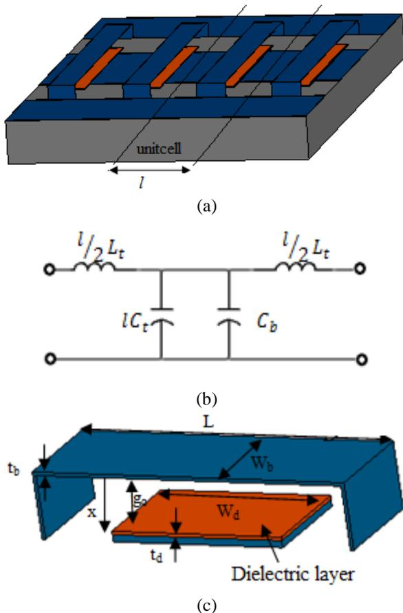
Fig. 2. a) Distributed MEMS transmission line (DMTL) b) simplified circuit model of unitcell c) MEMS bridge structure which modeled as capacitance of  $C_b$
