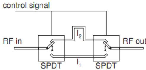
Fig. 1. Schematic of a conventional switched-line phase shifter
