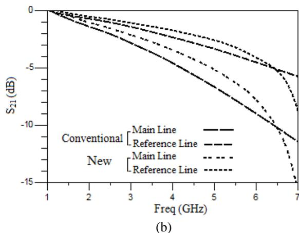
Fig.4. Scattering parameters of structures, (a)  $S_{11}$ , (b)  $S_{21}$
