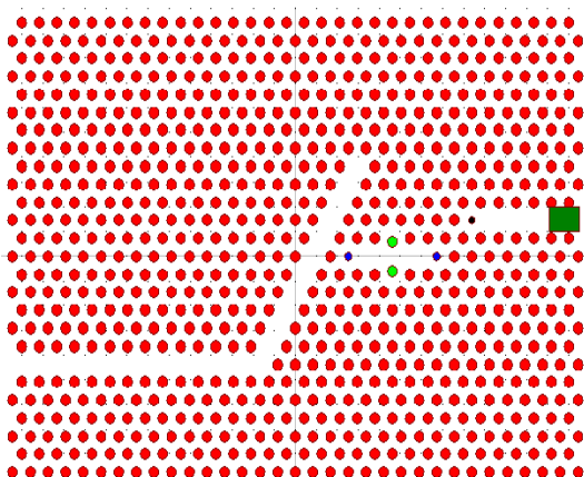
Fig. 3. Schematic structure of suggested base filter for two-channel demultiplexers of 2D photonic crystal
