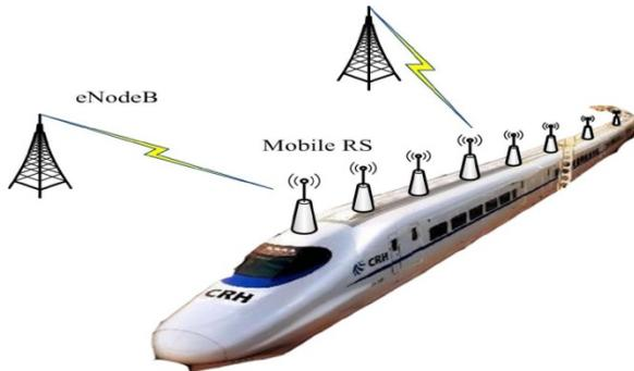
**Fig.1.** Illustration of the onboard transceivers in communication system of high-speed railway.
