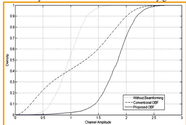
Figure 6. Impact of OBF on the distribution of channel amplitude.
