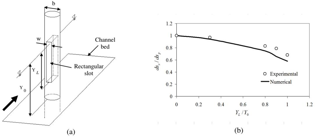
Fig. 4. (a) Geometric properties of slotted pier which was used in the study and (b) Variation of local scouring depth versus non-oriented slot length when the slot width is half of the pier diameter
