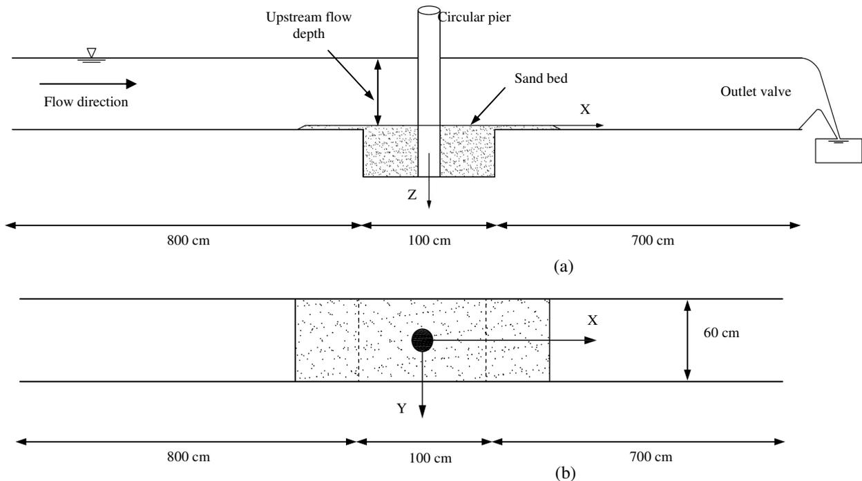
Fig. 1. Geometric properties of the flume in which experiments were done by Mia & Nago (2003); (a) longitudinal section, (b) plan view (not scaled).
