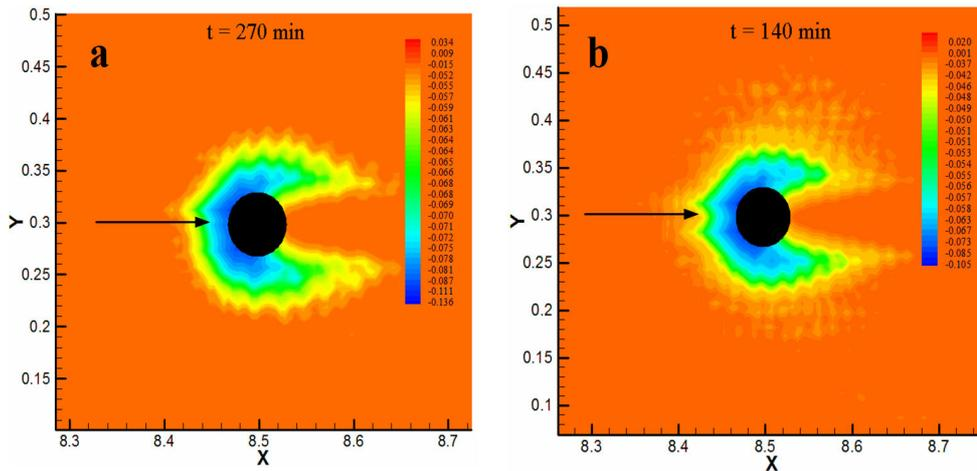
Fig. 3. (a) Bed changes in the vicinity of circular pier at the end of calibration and (b) verification stage
