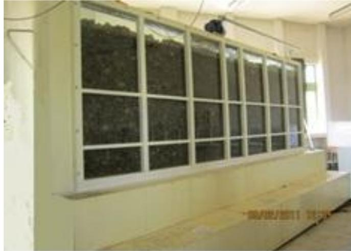
Fig. 3. Schematic of the permeameter.
