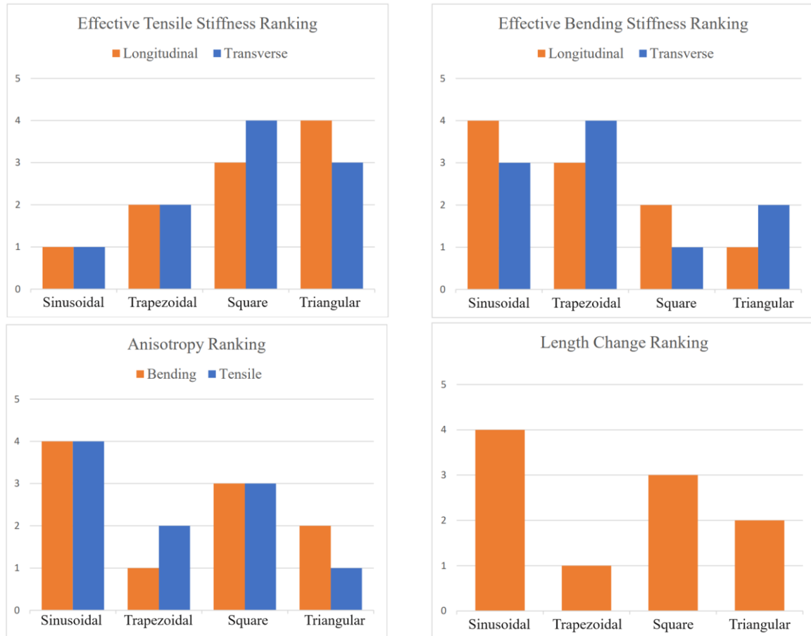
Fig. 4 Comparison of mechanical properties of corrugated shells.
