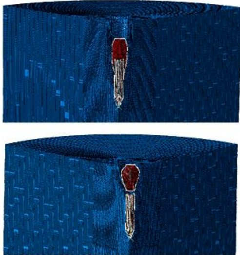
Fig. 10 Penetration and damage mechanism of the tungsten-core coated projectile in a 76 mm target, the friction coefficient between the coating and the target is 0 in the top figure and 0.4 in the bottom figure.
