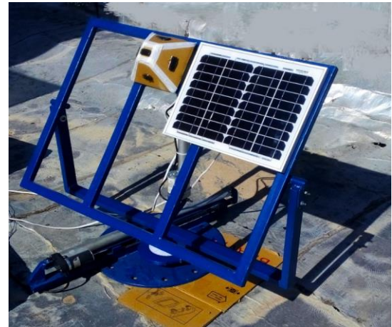
Fig. 1 The built structure with tracking equipment and solar panels
