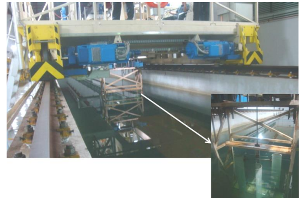
a) Experimental setting of fixed blades turbine.
