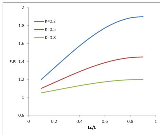
**Fig. 5** Frequency ratio versus normalized crack position
