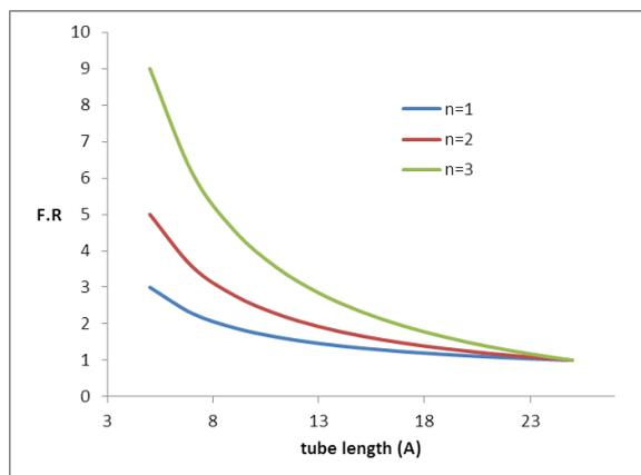
**Fig. 7** Frequency ratio versus tube length (A) for different mode number
