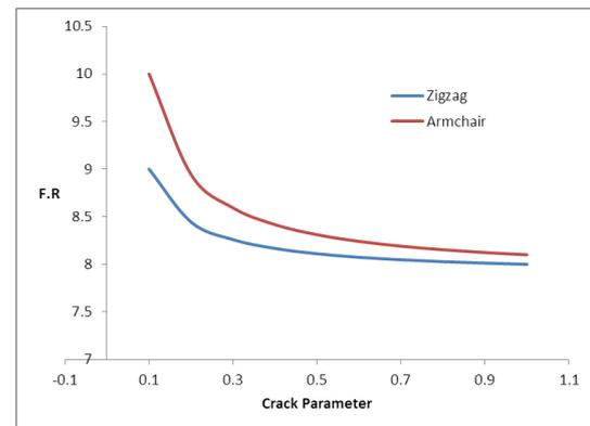
**Fig. 4** Natural frequency versus crack severity
