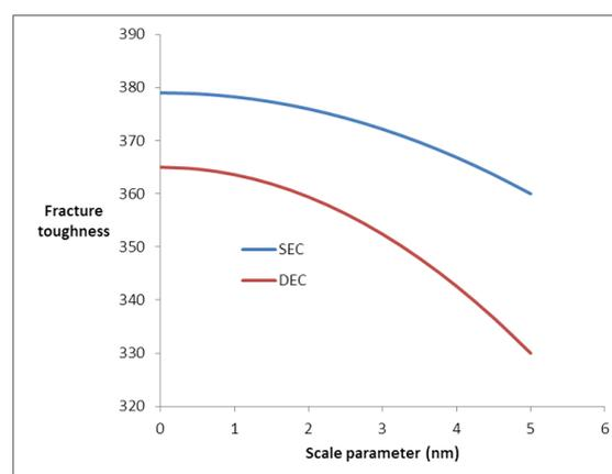
**Fig. 8** Fracture toughness ( $TPa\sqrt{nm}$ ) versus scale parameter for different crack type
