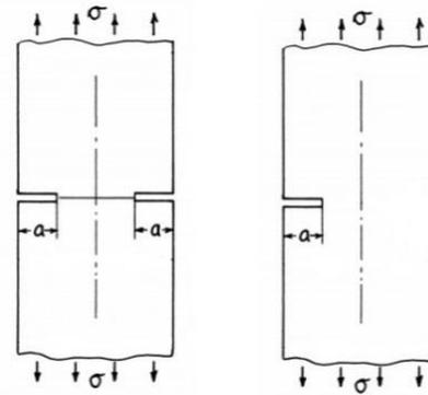
Fig. 3 SEC and DEC in axial loading of SWCNT
