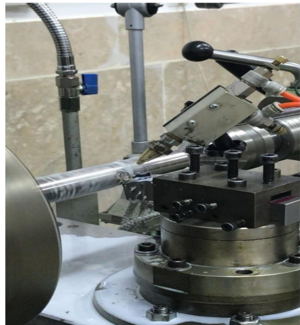
Fig. 3 Machining process of AISI 304 stainless steel workpiece using the MQL lubrication system
