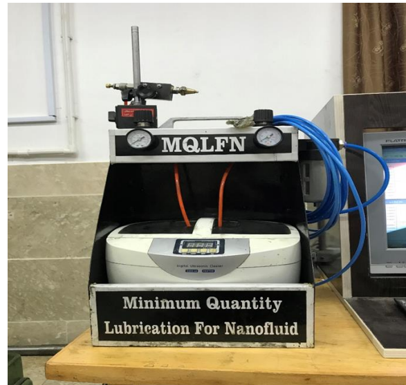
Fig. 2 Minimum quantity lubricant (MQL) device
