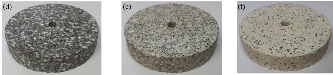
Fig. 1 (a) granite, (b) marble, (c) artificial stone made with resin, (d) artificial stone made with stone powder, (e) artificial stone made with lime and grey cement and (f) artificial stone made with lime and white cement.
