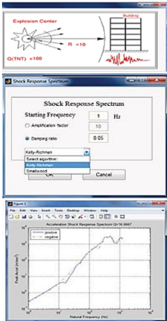
Fig. 10 Input information and results of shock response spectrum from the program
