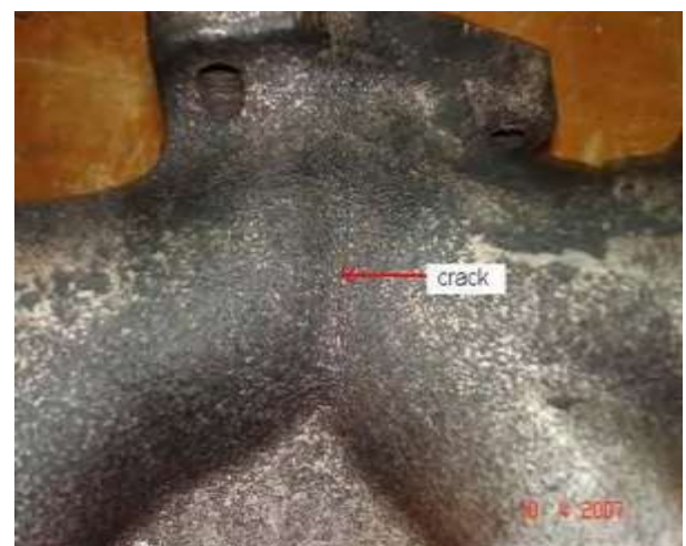
Fig. 10. The cracked exhaust manifold[33]
