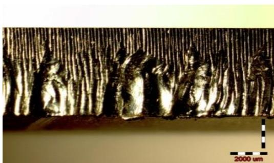
Fig. 29- Image of the Cutting Edge in 6mm Sheet under 3.5bar Pressure, 1.5m/min Cutting Speed and Power of 1500W
