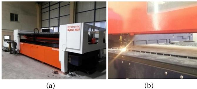
Fig. 3, (a) Bystronic Bystar-4025 Laser Cutting Equipment (b) Laser Cutting Equipment During Operation
