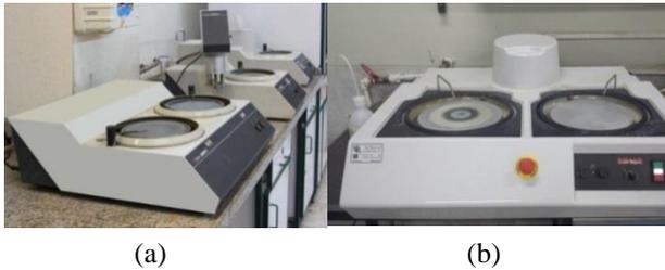
Fig. 2, (a) Sanding Equipment with Constant Water Flow, (b) Polishing Equipment Using in This Study.
