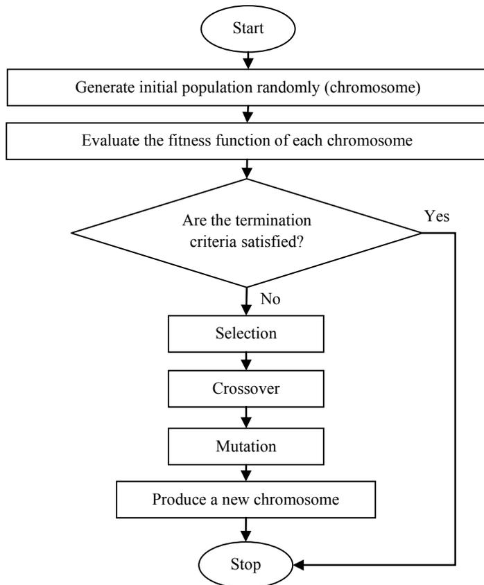
**Fig.2** Flowchart of the proposed GA optimization procedure.
