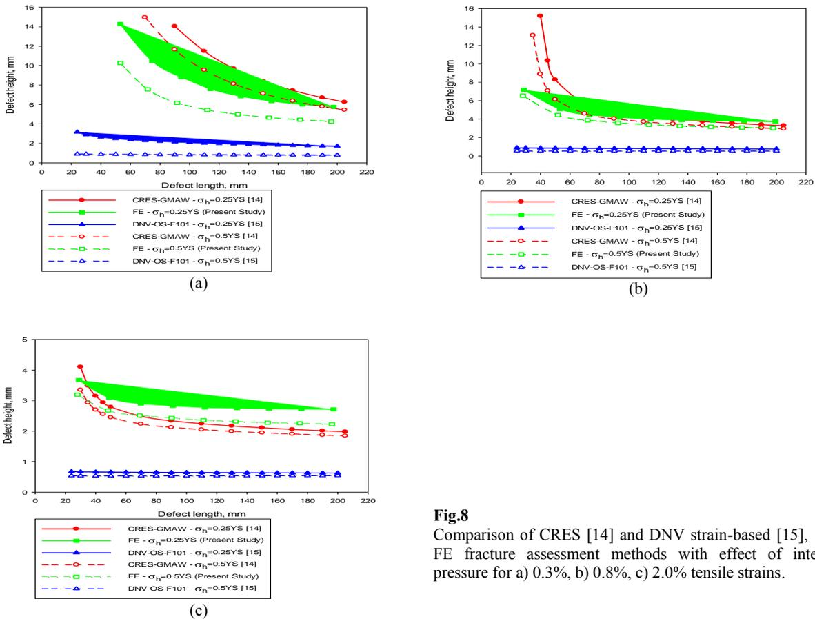
**Fig.8** Comparison of CRES [14] and DNV strain-based [15], and FE fracture assessment methods with effect of internal pressure for a) 0.3%, b) 0.8%, c) 2.0% tensile strains.
