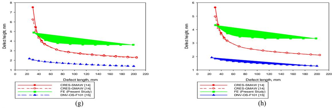
**Fig.7** Comparison of BS 7910 stress-based [9], FE, and DNV [15] and CRES [14] strain-based fracture assessment methods for a) 0.3%, b) 0.4%, c) 0.5%, d) 0.8%, e) 1.1%, f) 1.4%, g) 1.7%,h) 2.0% tensile strains.
