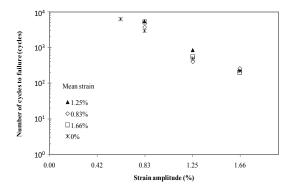
**Fig. 7** Changes in the fatigue lives of the specimens to the strain amplitude for CK45 steel.
