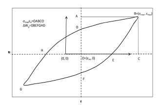
**Fig. 11**Graphical illumination of the SWT and energy damage parameter.
