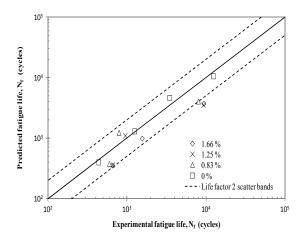
Fig. 13 Comparison of experimental and predicted fatigue lives based on SWT fatigue damage parameter,  $\sigma_{max}$   $\varepsilon_a$  for CK45 steel.
