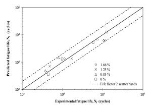
Fig. 15 Comparison of experimental and predicted fatigue lives based on SWT fatigue damage parameter,  $\sigma_{max}$   $\varepsilon_a$  for SS316 stainless steel.
