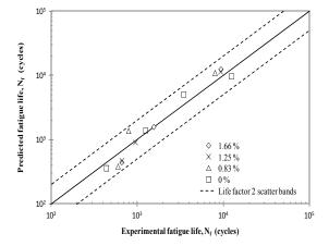
Fig. 12 Comparison of experimental and predicted fatigue lives based on energy fatigue damage parameter,  $\Delta W_p$  for CK45 steel.
