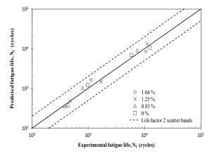
Fig. 14 Comparison of experimental and predicted fatigue lives based on energy fatigue damage parameter,  $\Delta W_p$  for SS316 stainless steel.
