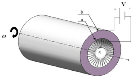
**Fig. 2** Hollow FGPM rotating circular shaft subject to uniform temperature field, uniform internal pressure, uniform external pressure and applied voltage  $V$ .
