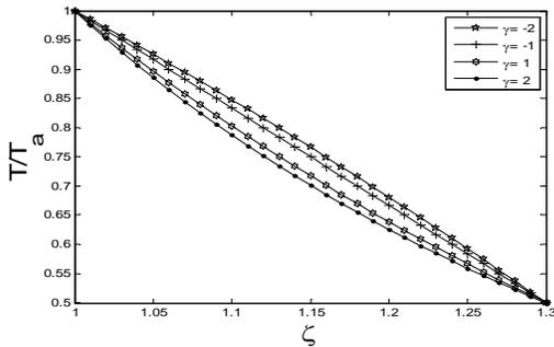
**Fig. 1** Temperature distribution of the FGPM cylinder for different values of  $\gamma$ .
