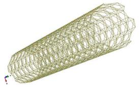
**Fig.3** Finite element model of a carbon nanotube.
