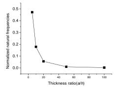
Fig. 2 Variation of natural frequencies of laminated composite clamped plates  $(0^0/90^0/0^0/90^0)$  with different thickness ratio (a/h).
