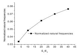
**Fig. 3** Variation of natural frequencies of laminated composite clamped plates  $(0^0/90^0/0^0/90^0)$  with different modular ratio  $(E_1/E_2)$ .
