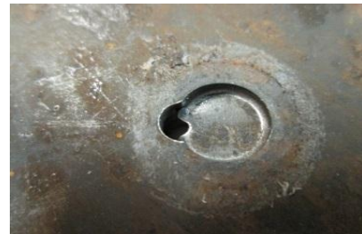
The hole with 5 mm diameter and 3 mm overlap l=12, d=5, y_{min}=0.9, y_{max}=1.08, \theta=7.73
