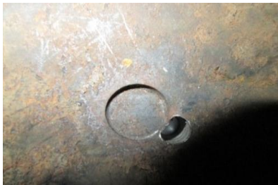
The hole with 5 mm diameter and 1 mm overlap l=14, d=5, y_{min}=0.9, y_{max}=1.7, \theta=5.07
