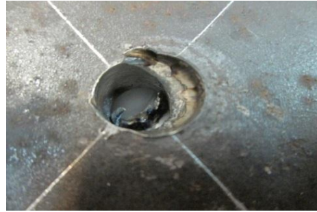
The hole with 9 mm diameter and 6 mm overlap l=13, d=9, y_{min}=1.7, y_{max}=2.5, \theta=11.3
