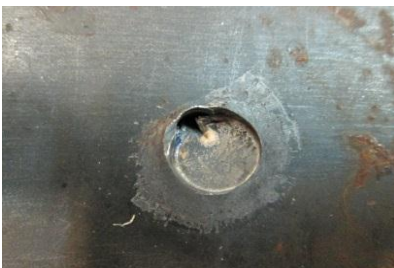
The hole with 5 mm diameter and 4.2 mm overlap l=10.8, d=5, y_{min}=1.1, y_{max}=2, \theta=8.82
