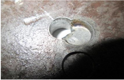
The hole with 9 mm diameter and 4 mm overlap l=15, d=9, y_{min}=1.2, y_{max}=2.3, \theta=10.38
