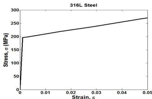
Fig.2 Stress-strain curve for 316L steel (Lee *et al.* [4])
