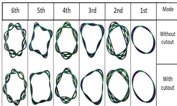
**Fig.4** Comparison of numerical analysis mode shapes in structure with and without cutout.
