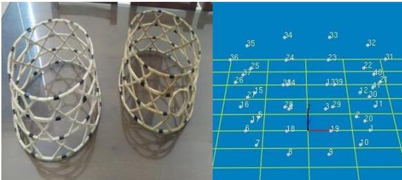
**Fig.3** Specified points in structures with and without cutout to run modal analysis.
