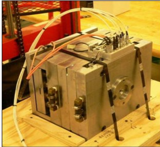
Fig. 2 Mold used to make the validation part and feed system.
