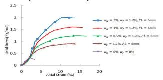
Fig. 8. Stress-strain curves of the soil mixture containing nanoclay, reinforced with fibers
