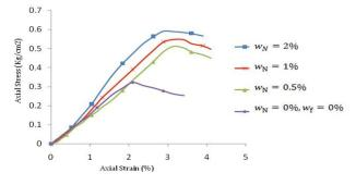
Fig. 7. The stress-strain curve of the soil-nanoclay mixture without the fibers
