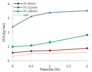
Fig. 10. Compressive strength of the soil-nanoclay with 0.6 weight percentage of fiber
