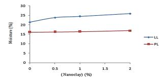
Fig. 2. Effect of adding Nanoclay on the Atterberg limits of the under study soil
