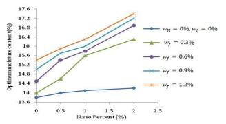
Fig. 5. The optimum moisture changes with the increase in the nanoclay content
