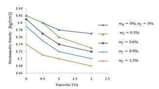
Fig. 4. The maximum dry density changes with the nanoclay content
