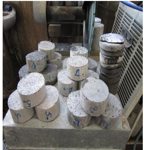
Figure 4. Cutting of 10*20 concrete cylinders to concrete slices smaller than 5*10 according to the standard.
