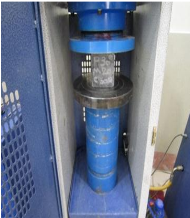
Figure 8. Sample failure with a 300-ton jack.
