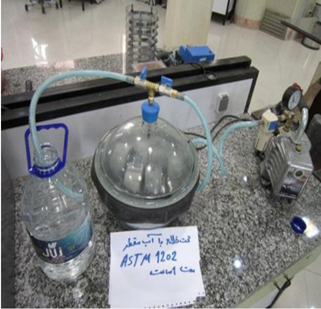
Figure 5. Concrete cutters 5 * 10, in vacuum machine.
