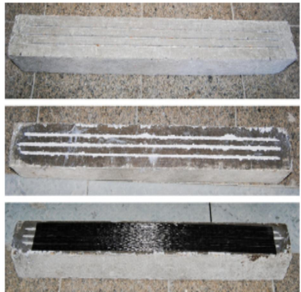
Figure5-Specimens strengthened with EBROG technique [4]
