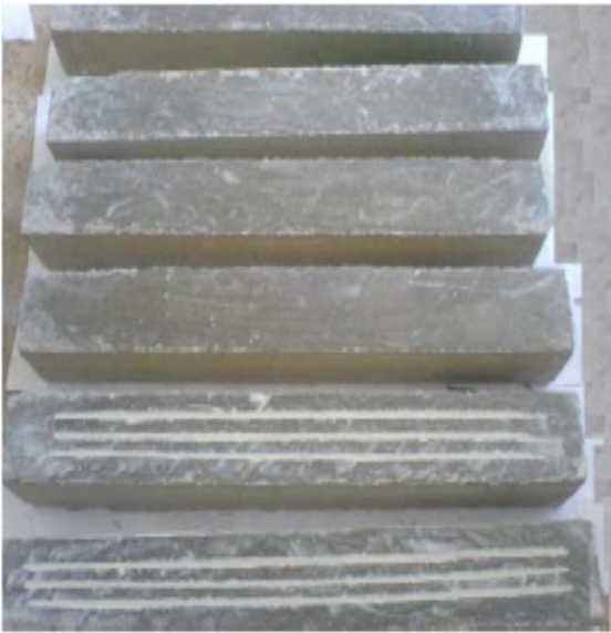
Figure2-EBR and EBROG methods [1] & [5]
