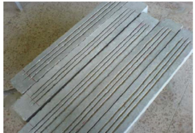
Figure1-Grooves at EBROG method [1] & [5]
