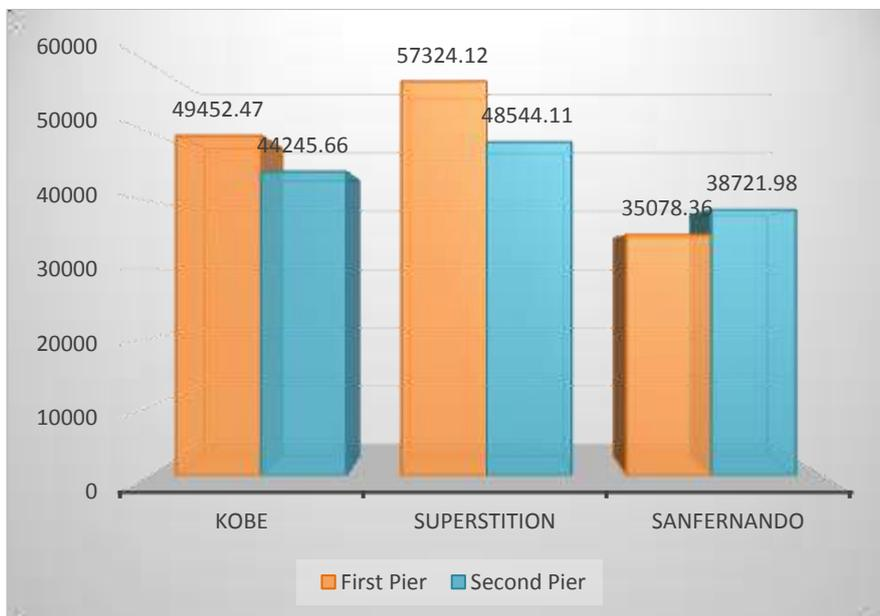
Fig.26. Maximum Axial Force of Bridge Piers Due to Records (KN)
