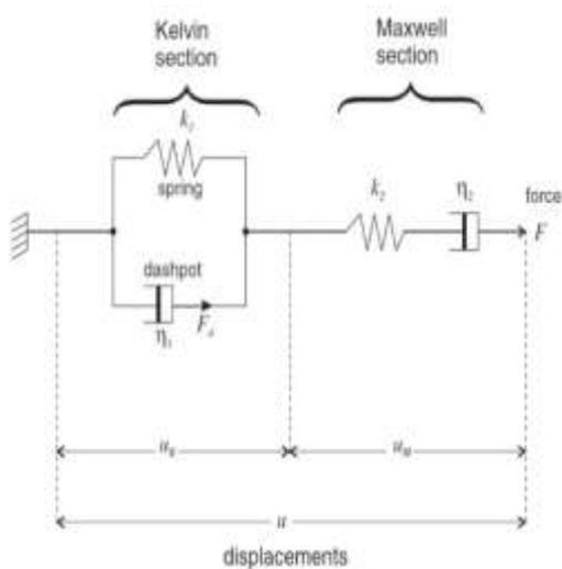
Fig.6. Schematic of Berger's behavioral model with definition of variables.
