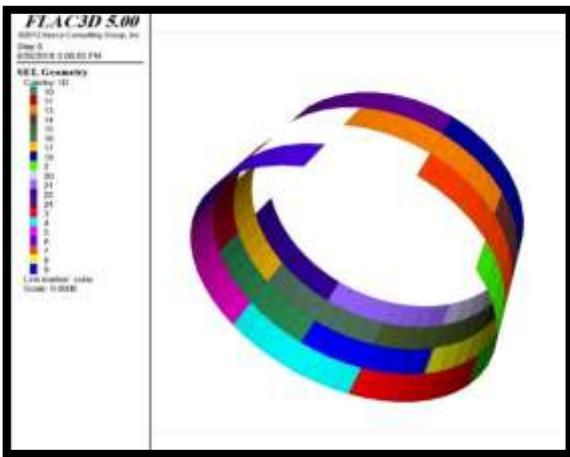
Fig.3. Displaying the segments and era of each loop compared to the previous loop in FLAC 3D software.
