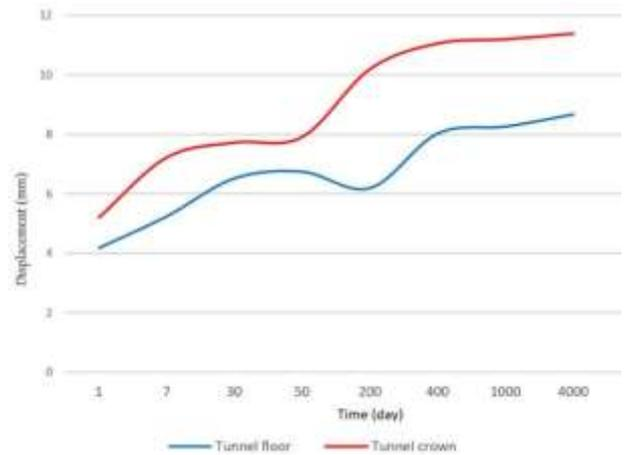
Fig.17. Comparison of tunnel crown and floor displacement.
