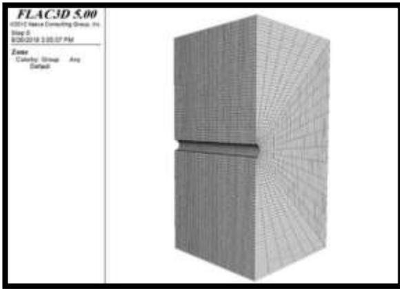
Fig.2. Half geometry modeled in FLAC 3D software.
