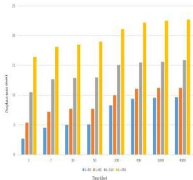
Fig.12. Comparison of displacement in different drilling depths considering the time dimension.
