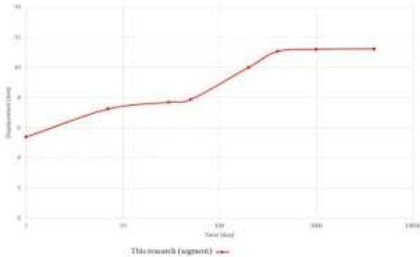
Fig.14. Displacement of segmental lining system.
