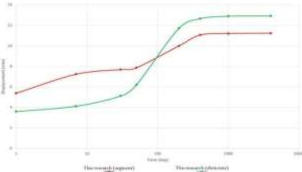
Fig.16. Comparison of displacement of segmental lining system with shotcrete.
