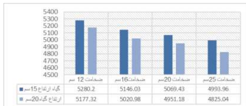
Diagram 6. Effect of bed layer height on annual heating consumption
