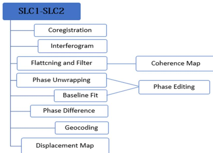
**Figure 1.** Intermetric method in remote sensing procedure
