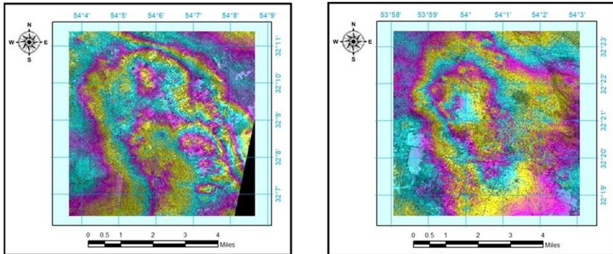
**Figure 4.** Finalized mapping with a mean land subsidence rate of 8 to 10 centimeters from 2015 to 2017 (Right: Ardakan, Left: sub-province Meybod sub-province) (<https://scihub.copernicus.eu>)
