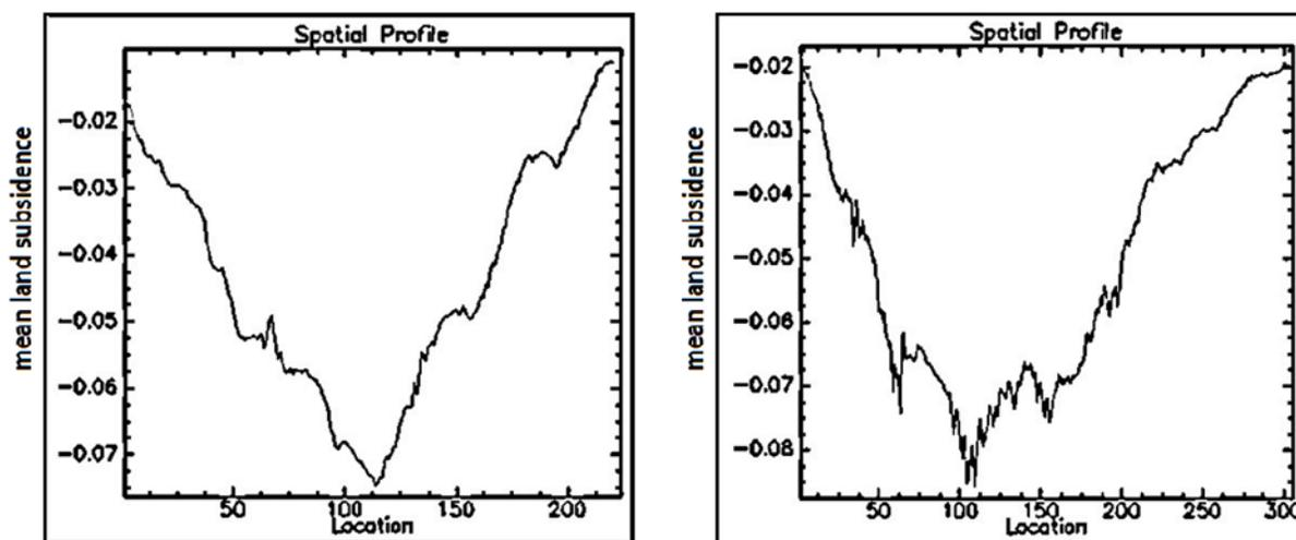
**Figure 5.** Longitudinal profile with a mean land subsidence rate of 8 to 10 centimeters from 2015 to 2017 (Right: Ardakan, Left: sub-province Meybod sub-province)
