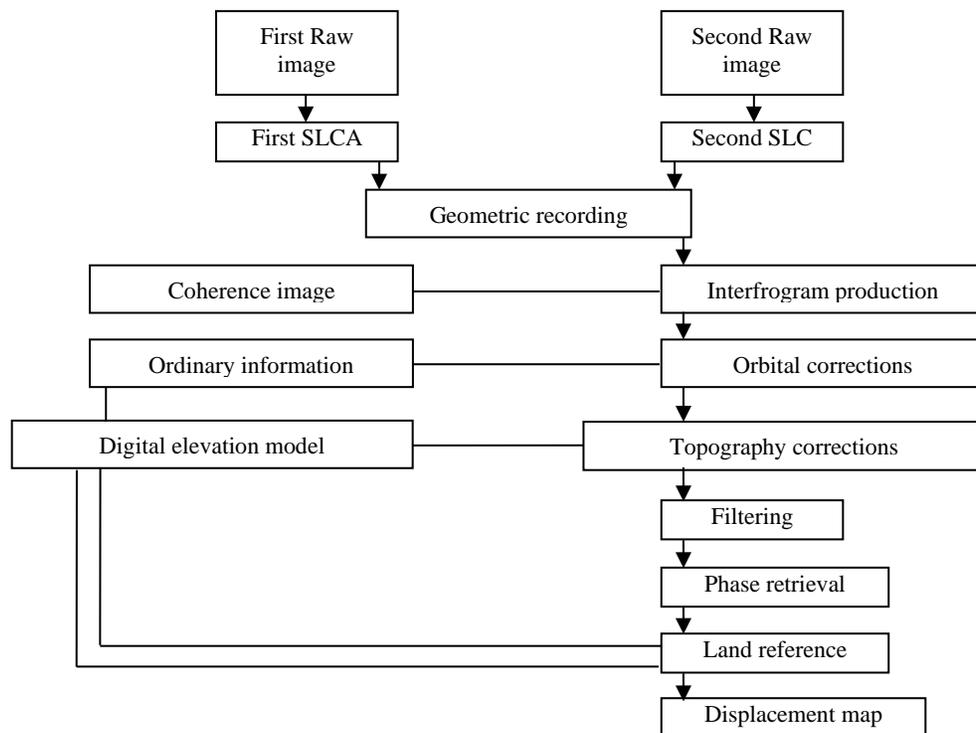
Figure 2. the interferometer Processing stages
