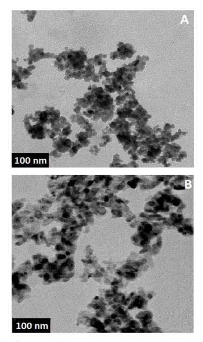
Fig. 4. TEM image of  $SnO_{2}\left(A\right)$  and C,N,S-tridoped  $SnO_{2}\left(B\right)$  nanoparticles.
