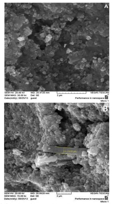
Fig. 3. SEM image of  $SnO_2$  (A) and C,N,S-tridoped  $SnO_2$  (B) nanoparticles.
