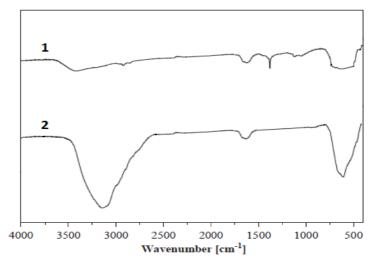
Fig. 2. FTIR spectra of SnO<sub>2</sub> (1) and C,N,S-tridoped SnO<sub>2</sub> (2) nanoparticles.
