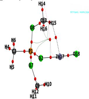
**Fig. 2.** DMMP connected to ZnO.
