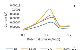
Fig. 6. a: Cyclic voltammetry of Ascorbic Acid, b: square wave voltammograms of Ascorbic Acid; The anodic peak currents  $(I_{pc})$  vividly increased in the square wave voltammograms compared to the Cyclic voltammetry; Experimental conditions:
