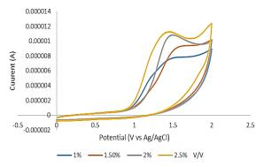
**Fig 4.** Cyclic voltammetry of *Ajwain* after spike; Experimental conditions: pH= 3.0,  $v= 0.1 \text{ Vs}^{-1}$  in different concentration, potential = 0 to 2.0 V, temperature = 25 °C, The cathodic peak current (*I<sub>pc</sub>*) increased with the increment thymol concentration.
