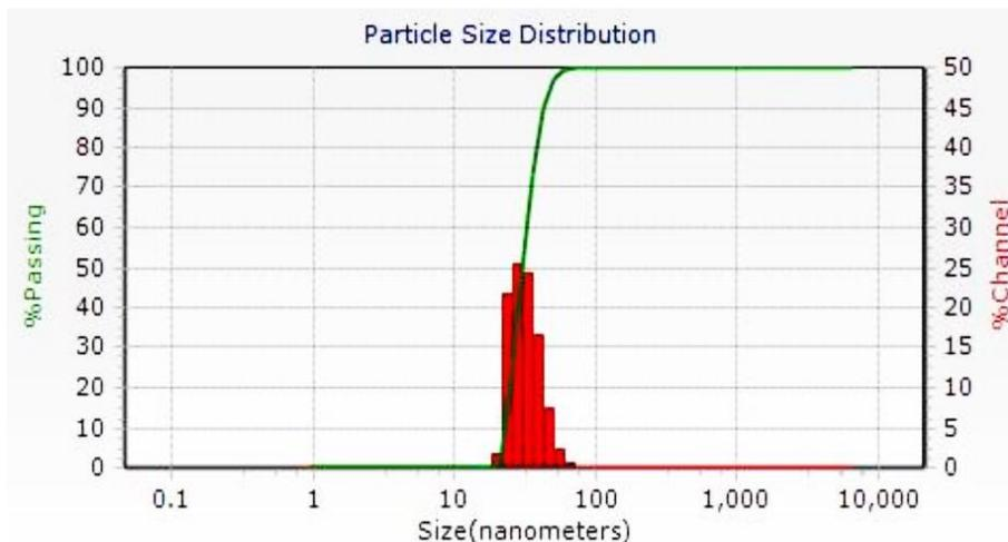
**Fig.4. Magnetic nano-fluid particles size distribution**
