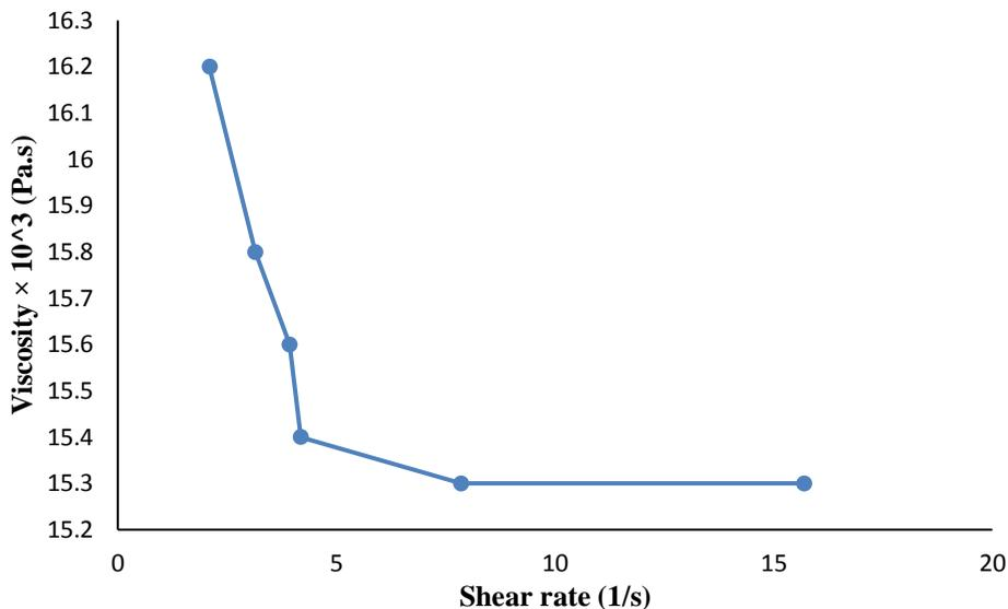
Fig.5. Viscosity values in terms of shear rate of the nano-fluid at a temperature of 20 °C.
