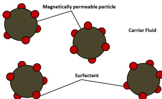
Fig.2. Magnetic nano-particles with surfactant
